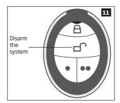
To verify if the system has been successfully armed, do not release the *Arm the system* keyfob button and wait for the 3 short keyfob buzzer's beeps/indicator's flashes indicating the successfully carried out command. The long beep/flash indicates the unsuccessful command.
