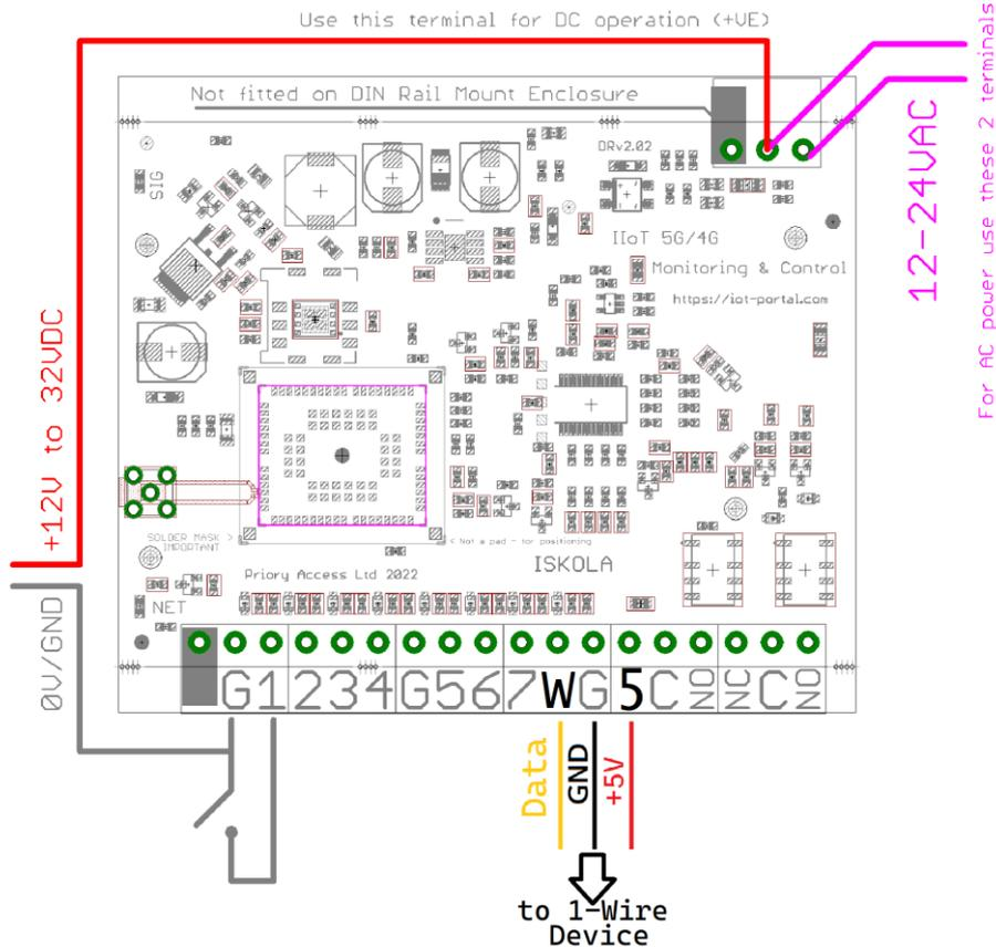
The TR5 needs to scan the 1-Wire bus in order to use any devices connected to the 1-Wire input. To do this, go to the 'Live Screen' > 'Tools' (Blue Button) > '1-Wire'.
