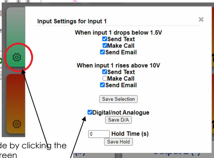
Choose between analogue and digital mode by clicking the gear wheel on the input card on the Live Screen
