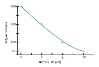
Note: Battery life is dependent on many factors, including daily activations, time used per activation, radar range and external conditions.
