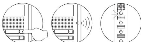
Press the door panel push button that will call this monitor. At this moment the door panel will reproduce a sound and the monitor led will blink.
