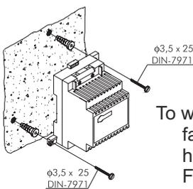
Install the transformer in a dry and protected location. Please note that current regulations stipulate that the transformer must be protected by a circuit breaker.
