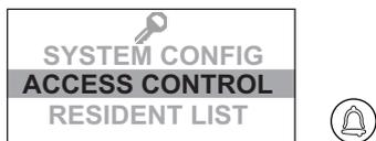
To access the access control menu, follow the steps described on p. 129 and press **A** when the ACCESS CONTROL message lights up.
