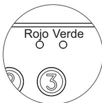
The self-testing LEDs are located on the top right-hand side of the front of the module.
