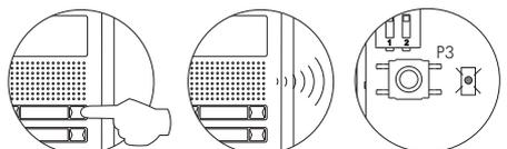
Press the door panel push button that will call this telephone. At this moment, the door panel and the handset will emit a number of tones (the LED on the telephone will blink slowly).
