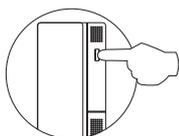
With the door release push button pressed, pick up the telephone's handset.
