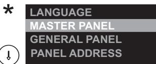
Determines whether the door panel is master or slave. Each system must have only one master door panel; the others must be slaves. In systems with a general entrance door panel, set one door panel from each building as the master. To change the value, press **Ⓜ**.
