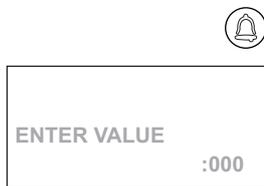
To change the value, press **Ⓜ** and the message ENTER VALUE will appear; enter the building code using the numeric keypad and confirm by pressing **Ⓜ**. Press **Ⓢ** to restore the previous value.
