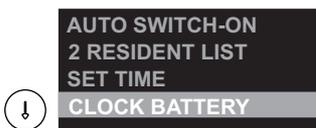
Enables the internal battery to be activated for the door panel to keep time. If the option is activated, the system will keep time even when the device has been switched off for an extended period of time. To change, press **Ⓜ**.
