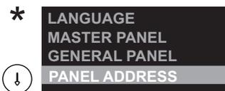
Determines the building code. In buildings with more than one door panel, set the same code for all of the panels; in systems with a general entrance door panel, set code 0 for the general entrance door panel and a different code for each inner door panel (between 1 and 255).
