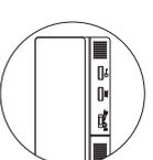
To programme the telephone as the *Master*, press the hang up button (the LED will go out). Close the telephone.
