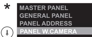
Determines whether the door panel is an electronic audio or video door entry system. To change the value, press **Ⓜ**.
