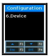
The description of function buttons such as F1, F2, F3, and F4 is in numerical order on the bottom of the screen as shown above. Go up and down the screen, you can press [ENT](F4) button to select the desired menu, or press [ESC] (F3) for more than 2 seconds to return to the upper menu.
