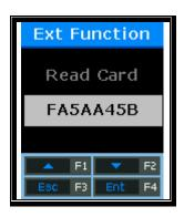
This is an additional function regardless of the terminal environment setting. In the case of the terminal that the card reader is added, the card number can be checked for card registration via the server. Place the card on this screen, and the card number will be displayed on the LCD.
