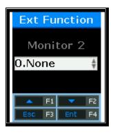
Set when connecting an external contact to DM1. (When using a motor lock, set to 1 or 2.) Default Setting: '0.None'
