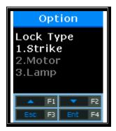
Set to '1' when the terminal is connected to the strike type or automatic door, and '2' when it is connected to the motor lock.
