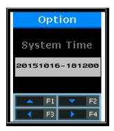
The current time of the terminal is displayed in the order of "2009:Year, 08:Month, 01:Day, 21:Hour, 18:Min, 06:Sec". To modify, move to the desired position using  $[\leftarrow][\rightarrow]$  buttons, and modify the existing values using  $[\uparrow][\downarrow]$  buttons.
