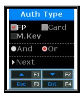
By using [↑][↓] buttons, select the authentication method and "And" or "Or", and press "Next" button.
