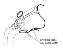
9. Quickly remove service cable and thread operating cable into unit until cable bottoms out and alarm stops sounding. Retain service cable for future maintenance.
