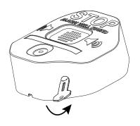
2. To remove cover from base, push with thumb to separate (as shown)
